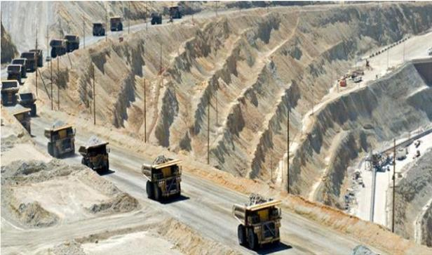
Open-pit mining - involves removing the layers of sand and rock found just above the kimberlite.
